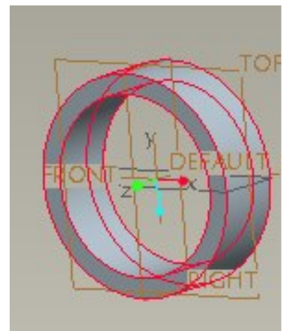
The basic 3D form, ready to have edges rounded and cut some holes
