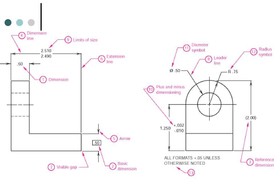
• Limits of size is the largest acceptable size and the minimum acceptable size of a feature.
