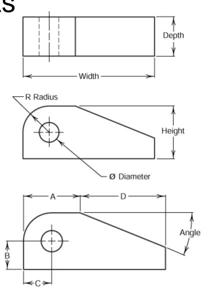
• Rectangular coordinate dimensioning, a base line (or datum line) is established for each coordinate direction, and all dimensions specified with respect to these baselines. This is also known as datum dimensioning, or baseline dimensioning. All dimensions are calculated as X and Y distances from an *origin point*, usually placed at the lower left corner of the part.
