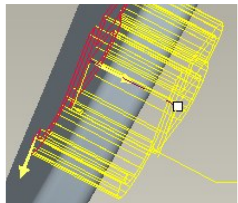
The text extruded through the key fob, ready to remove material
