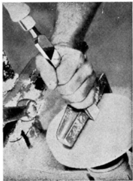
Fig. 17.12 Facing the Work with a Square-Nosed Chisel. A skew chisel could also be used.
