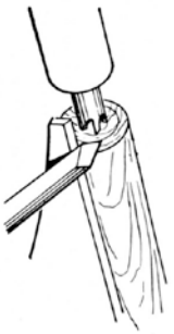
Fig. 17:23 Squaring the End of the Stock with a Skew Chisel
