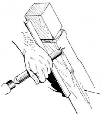
Fig. 17.17 Square-Nosed Turning Chisel Pick up second cut
