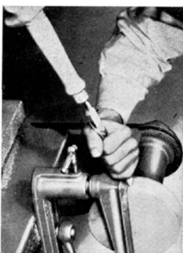
Fig. 17.10 Roughing the Work to Size with a Gouge
