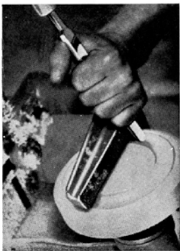
Fig. 17.12 Facing the Work with a Square-Nosed Chisel. A skew chisel could also be used.
