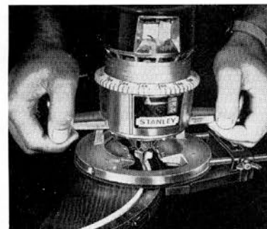
Fig. 18:8 Wood Section Added to Guide
