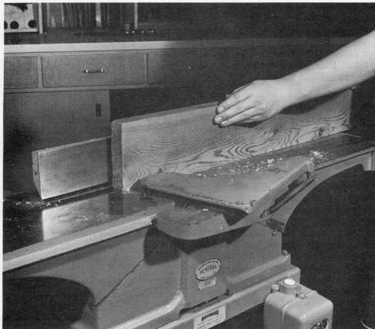
Fig. 20:4 Jointer with Spring Guard
