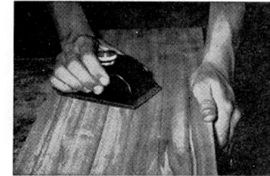
Fig. 23:8 Sanding with Tungsten Carbide
