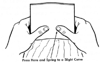
Fig. 23:7 Method of Holding a Hand Scraper
