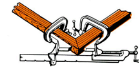
Fig. 13:7 Clamping a Flat Mitre Joint Using Clamp Blocks
