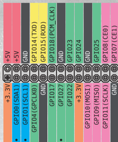
Raspberry Pi GPIO connector (P1) pinout
